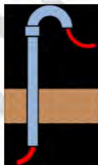
Pipe arrangement to exit out of the ground
